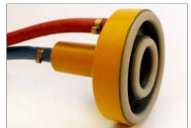
Two-chamber vacuum cell with sealing rings
